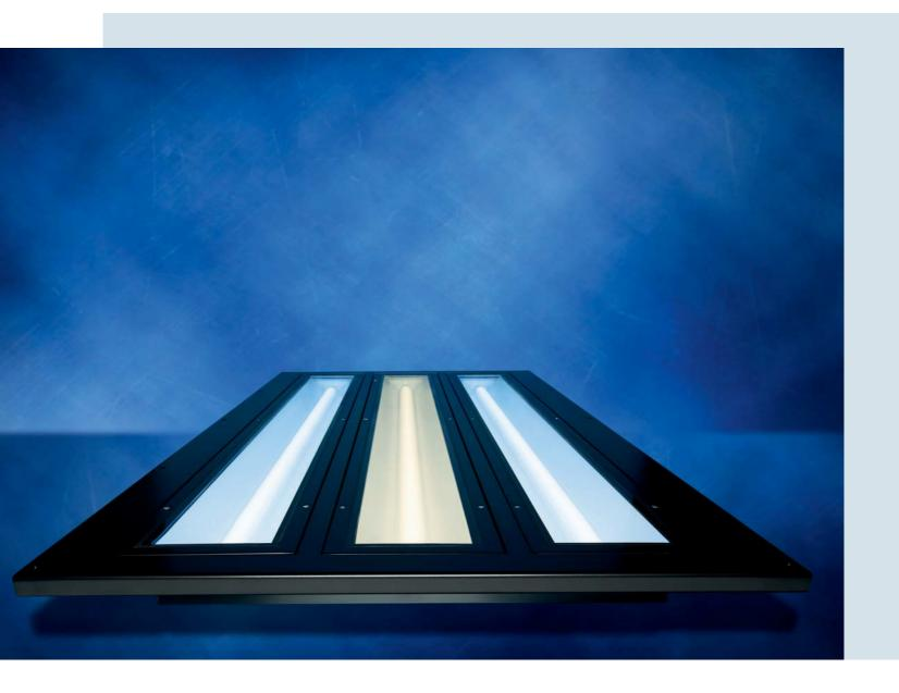
JUNG JBG floor luminaires are underfloor lights featuring 1, 2 or 3 LED strings, designed for inspecting surfaces of various characteristics. The laminated safety glass pane (VSG) is bonded to aframe, which is screwed into the lamp housing. In combination with JKL surface inspection lights it is possible to create a complete paintwork inspection system.
